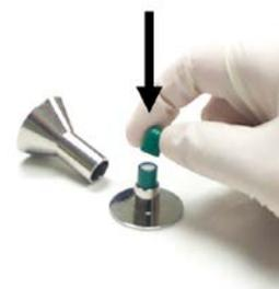
6. Place the capsule's cap onto the body of the capsule, pressing firmly to lock. Remove the filled capsule from the base.
