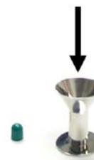
3. Dose a pre-measured amount of powder into the capsule through the funnel, **or** put the assembly on a precision balance, tare it, and dose the powder into the capsule through the funnel.
